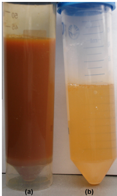
Fig. 4. Photographs of maghemite nanoparticles, stored three days in water, as demonstration of their excellent colloidal behaviour: water dispersions with maghemite nanoparticle concentrations of (a) 3.2 mg l −1 and (b) 0.1 mg l −1 .
