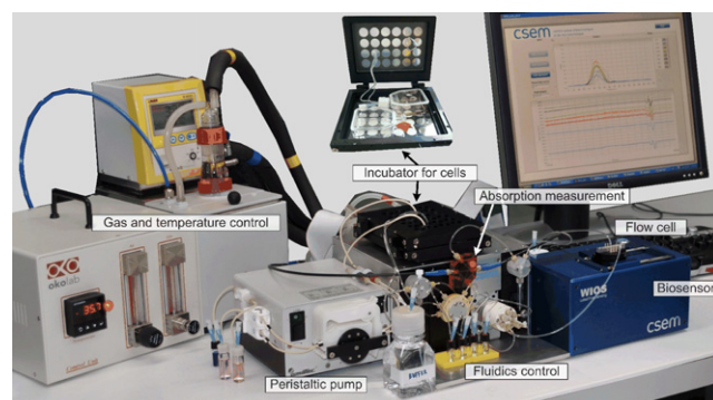
Fig. 1. The integrated platform allows in-line monitoring of cell cultures for the assessment of cellular toxicity of external agents. The elements of the platform comprise the cell culture unit, with its incubator (inset: measurement and reference cell culture flasks in incubator), the absorbance flow cell for cell proliferation measurement with AB, and the WIOS device with associated fluidics for cytokine detection with the immunoassay.
