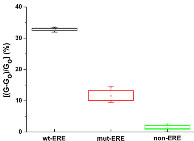
Fig. 4. Specificity of ER \alpha with various EREs immobilized on the SAM-assisted SiNW biosensor surface.
