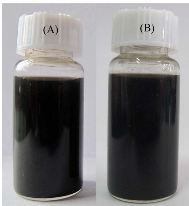
Fig. 2. Photographs of GNS-CNS dispersed in water (1 mg/mL) after ultrasonication 1 h (A) and stand for 30 days (B).
