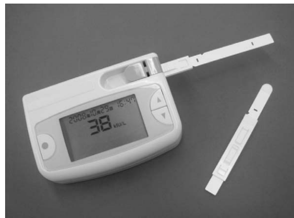
Figure 1 Portable sAA biosensor comprising of hand-held reader and disposable collector strip.
