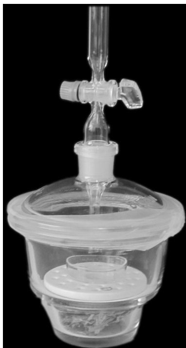
Fig. 2. The Conway chamber used for assaying sperm toxicants emitted by vinyl tiles of buildings.
