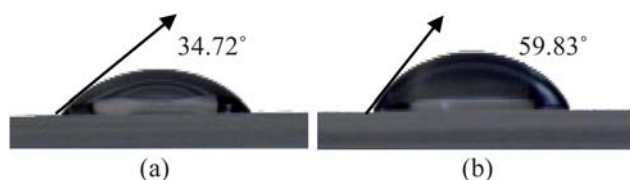
Fig. 3 Water contact angles for cleaned glass slide. (a) 34.72° before 3-GPS modification and (b) 59.83° after 3-GPS modification.
