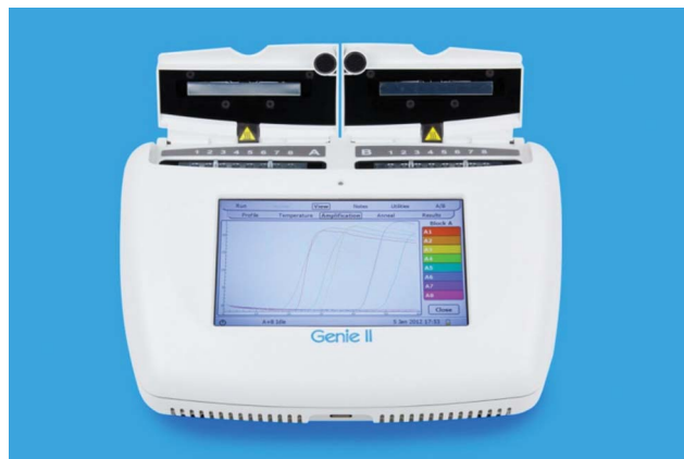
Fig. 1 Genie II (OptiGene, Horsham, UK) platform for fluorescence detection of isothermal amplification reactions allows isothermal reactions to be run in parallel with real-time fluorometric detection. (Image used with permission of OptiGene).
