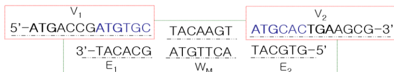
Figure 4. An example of path creation containing a weight.
